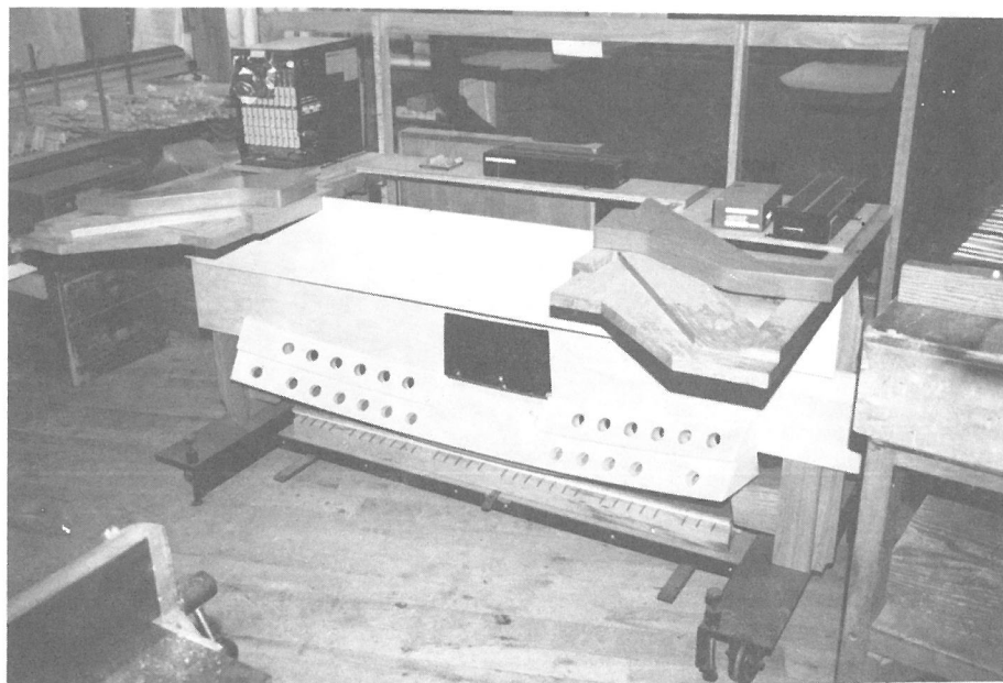
THE CONSOLE OF THE NEW ORGAN is beginning to take shape at the Casavant workshop in Canada. Some of the console's electronic components are in the background.
