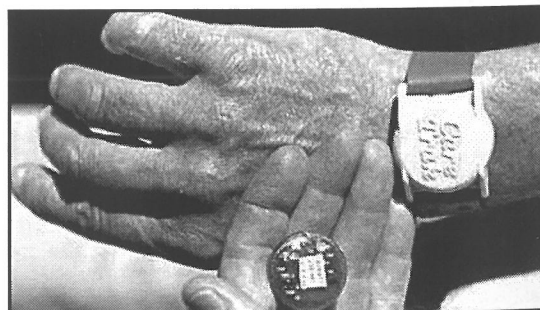
A signal is sent from this device, which is worn like a wristwatch, to alert searchers of a lost individual.
